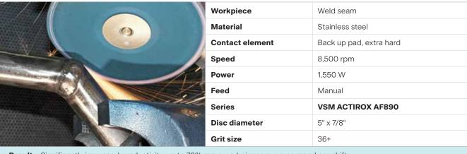
> Result: Significantly increased productivity, up to 70% more workpieces are processed per shift
