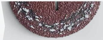
Fiber disc clogged with aluminum chips
