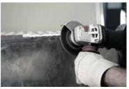
Removing welded seams
