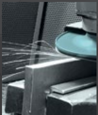
Weld seam preparation
