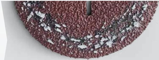
Fiber disc clogged with aluminum chips
