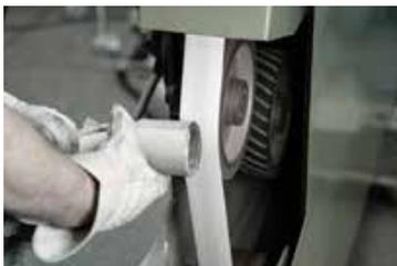
Grinding of cast parts
