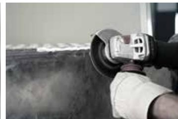
Removing welded seams
