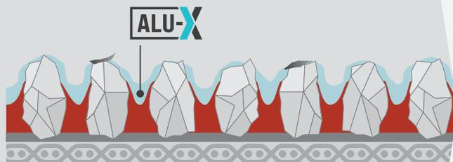
The VSM ALU-X additional layer significantly reduces adhesion; the abrasive can be used for longer.
