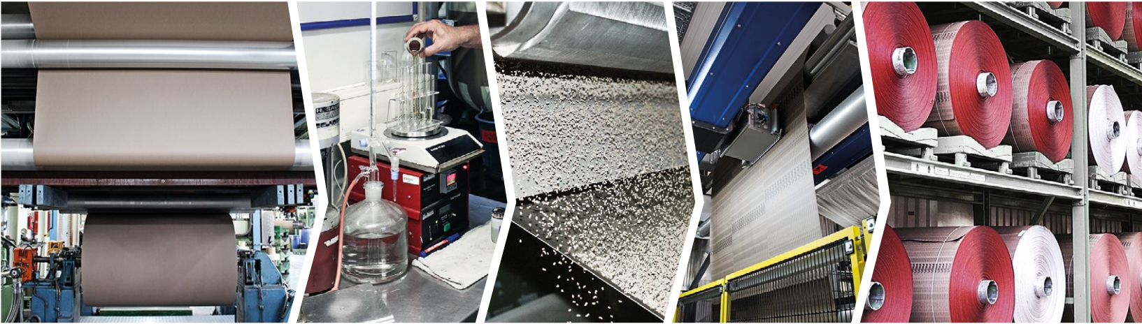
Finishing of backing materials Resin production Production of abrasive grain Coating and spreading Basic goods
